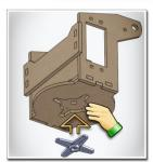
USE #2-56 1/4 INCH (6MM) WOOD 13 SCREWS TO MOUNT SERVO HORN
