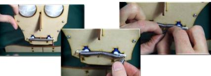
GIVE **CLEARANCE FOR USB** CONNECTOR TO PIVOT THROUGH
