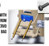
FOR ACRYLIC — USE #2 NUTS, LOCK **WASHERS AND** 5/16" (8 MM) **SCREWS**
