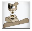
HOLD MOTOR WITH HAND WHILE 17 PRESSING NECK SERVO HORN **ONTO MOTOR**
